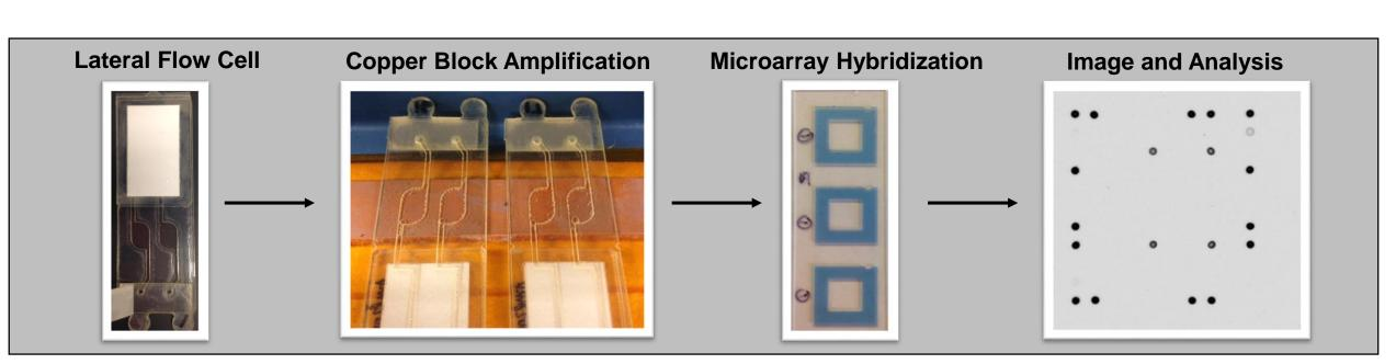
Figure 2: Amplification workflow for Akonni's TruArray platform. Samples are loaded into a lateral flow cell and placed on a flat block modified with a copper strip to isolate heat transfer. After asymmetric PCR amplification, PCR products are removed and cy3-labeled amplicons are hybridized to a microarray containing target-specific probes. Arrays are washed, imaged and analyzed.
